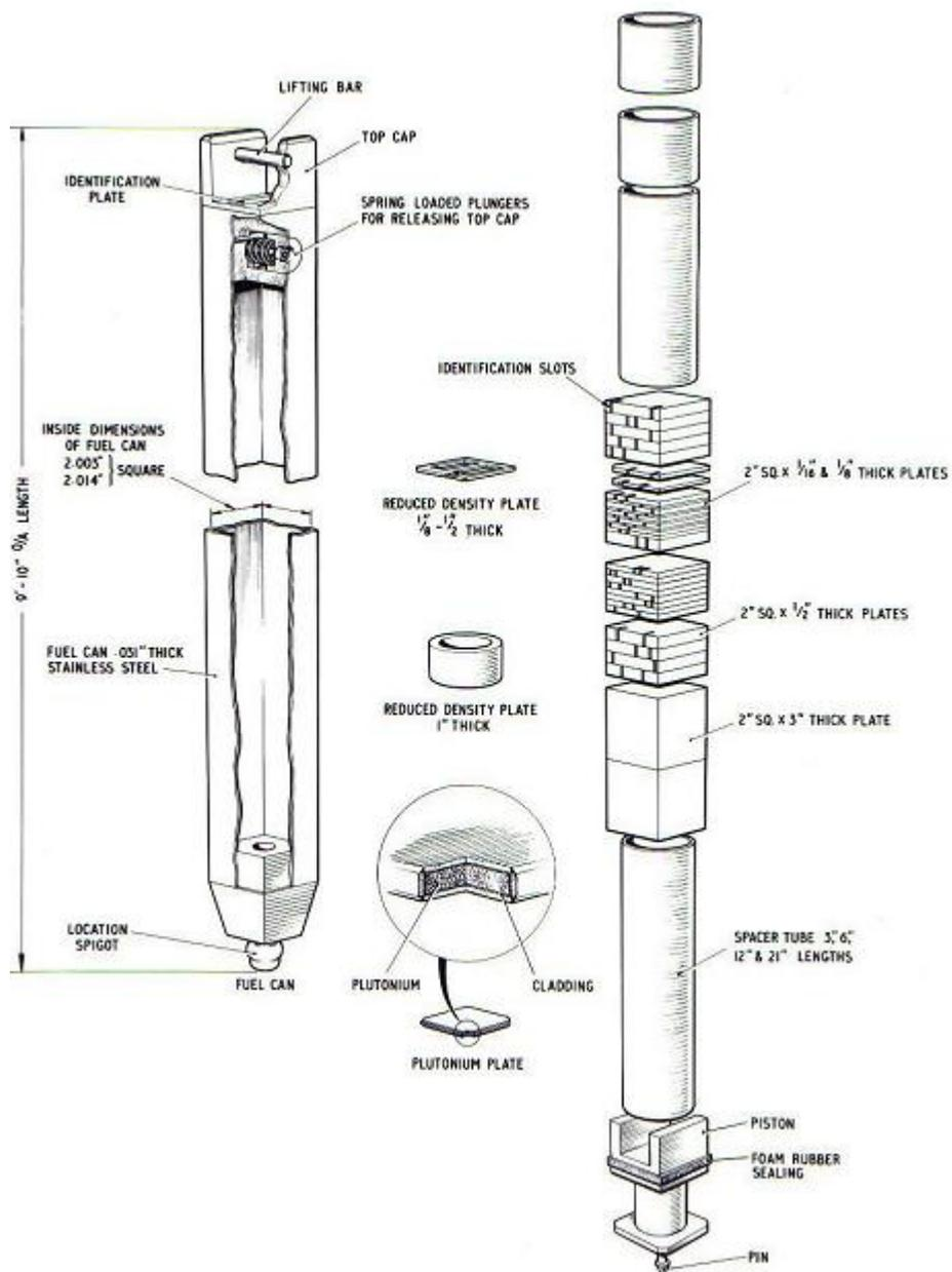
**Figure 4 Diagram of a Fuel Element Containing Materials in Plate Form**
