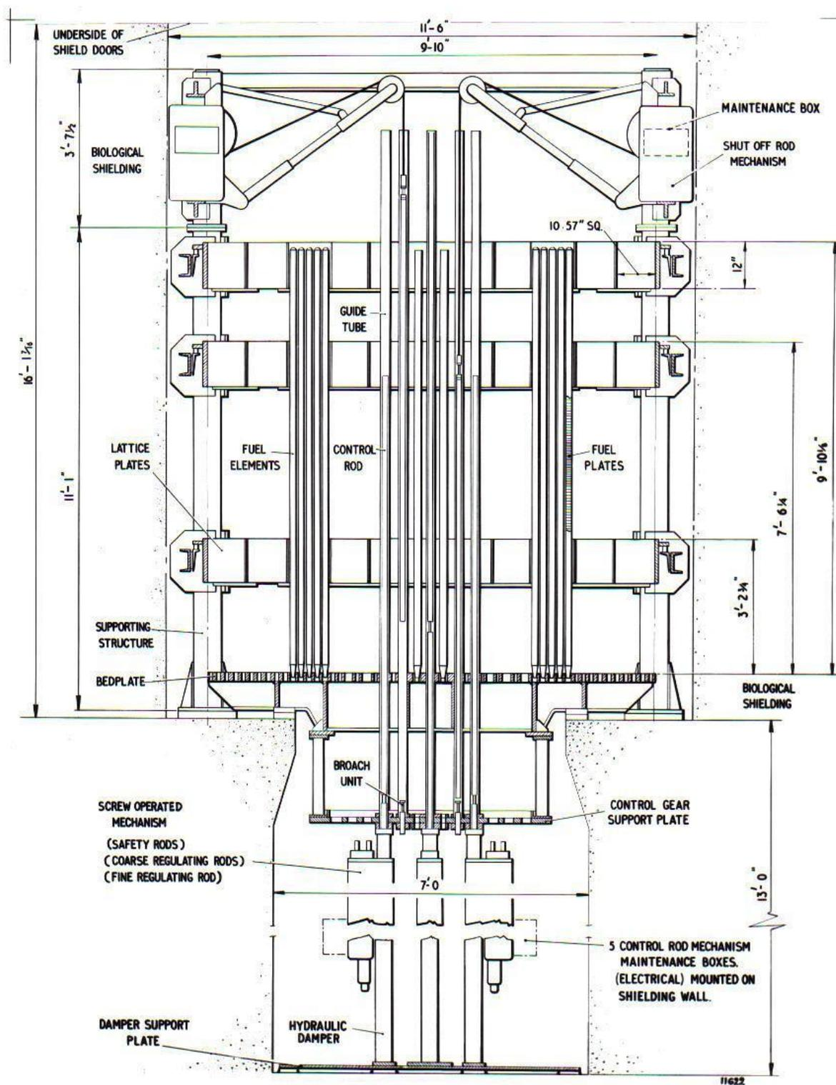
Figure 3 Vertical Sectional View of the ZEBRA Facility.
