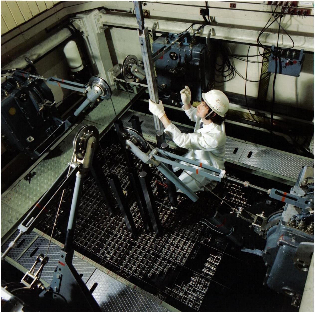
**Figure 2 View of an Element being Loaded into a ZEBRA Assembly.**
