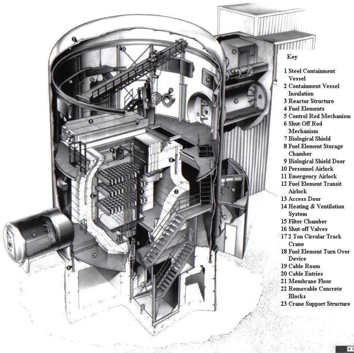
**Figure 1 A Perspective View of the ZEBRA Critical Assembly Facility.**
